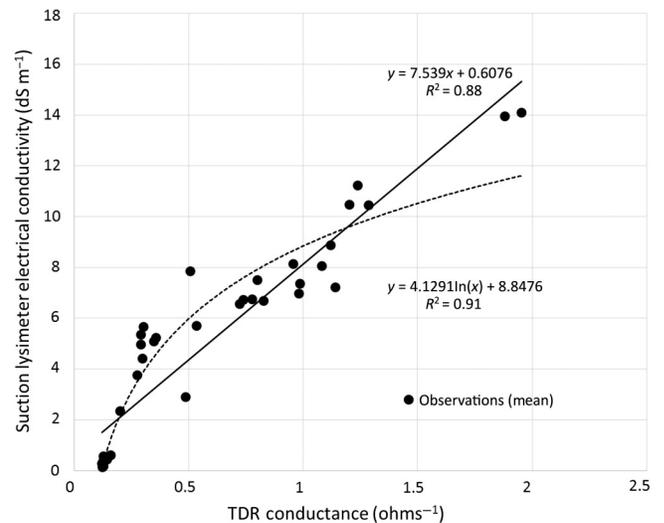
done using the [Rhoades et al. \(1989\)](#) model (Fig. 4), while the [Hilhorst \(2000\)](#) model was used for GS3 probe data (Fig. 5), as these approaches had given the best results using the raw data for each individual instrument
